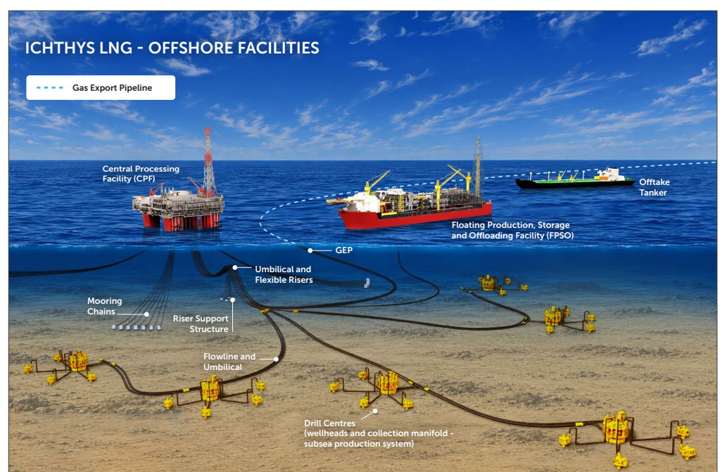
Figure 3: Ichthys LNG subsea production system overview.
