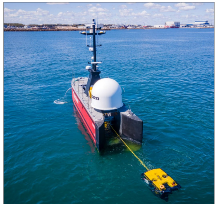
Figure 3: Example of an uncrewed survey vessel towing an ROV.
